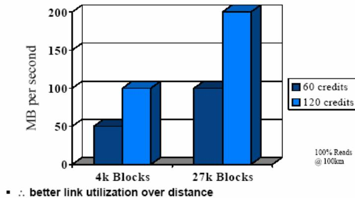
**Figure 3. Data rates based on buffer to buffer credits**
