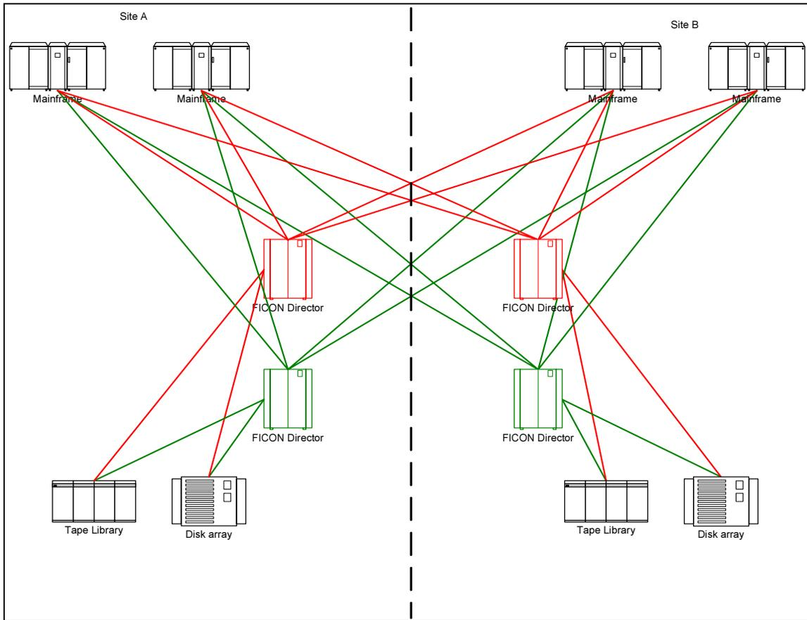
**Figure 1 – Two-Site, Non-cascaded FICON environment**
