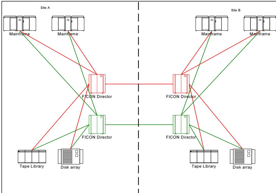
**Figure 2 – Two-Site, Cascaded FICON environment**
